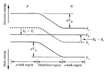
2. (a) In the depletion approximation for the pn diode, why do the holes and electrons not continue to diffuse until the all the electrons and holes carrier concentrations are evenly dispersed throughout the device? (b) In the bulk regions of a pn diode, what is the value of the electric field. Explain your answer.
